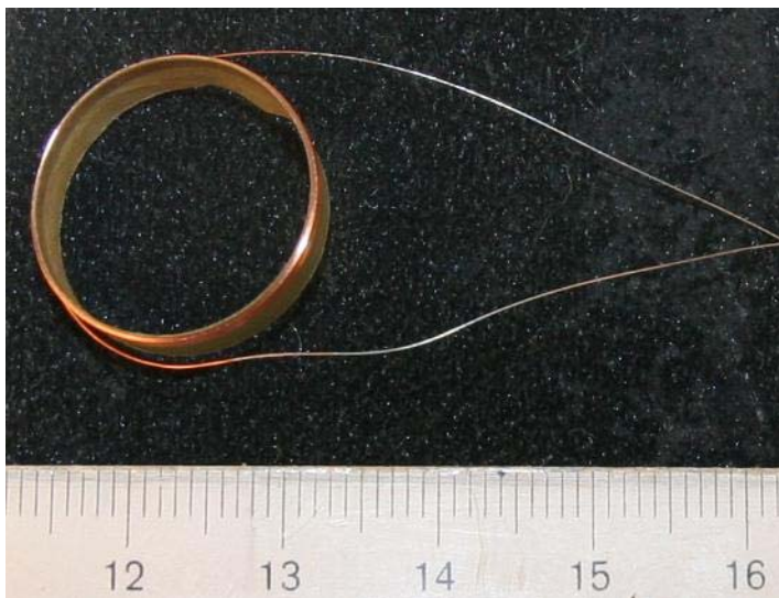
Figure 2: A voice-coil with a pre-tinned enamelled CCAW
