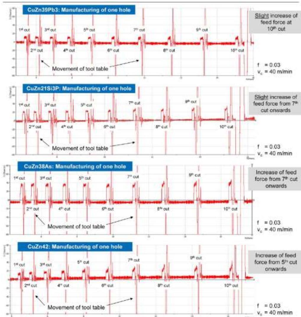
Fig. 11: Comparison at feed forces –  $v_c = 40$  m/min,  $f = 0.03$  mm
