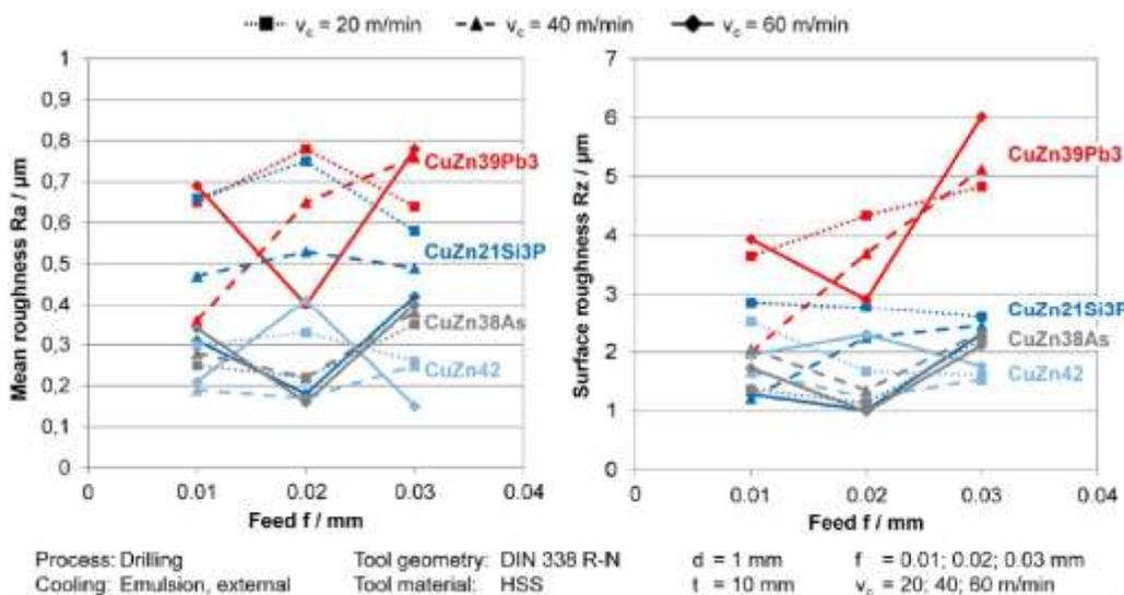
Fig. 15: Comparison of surface roughness
