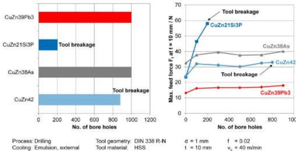
Fig. 16: Comparison of tool wear and maximum feed force
