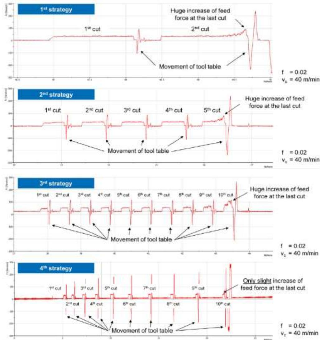
Fig. 5: Comparison of drilling strategies with respect to feed forces when drilling CuZn38As
