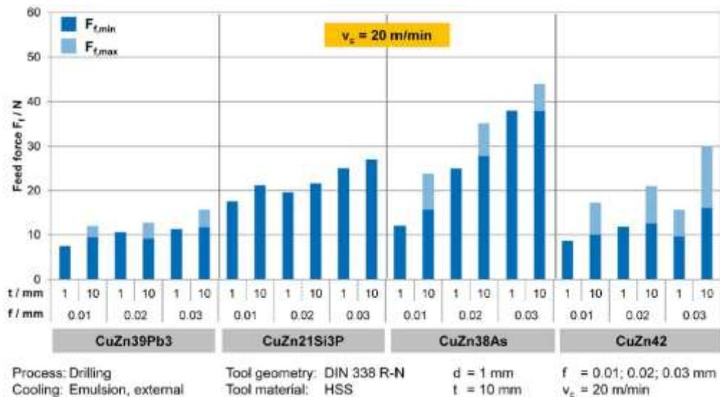
Fig. 12: Comparison of feed force at a cutting speed  $V_c$  of  $20 \text{ m/min}$
