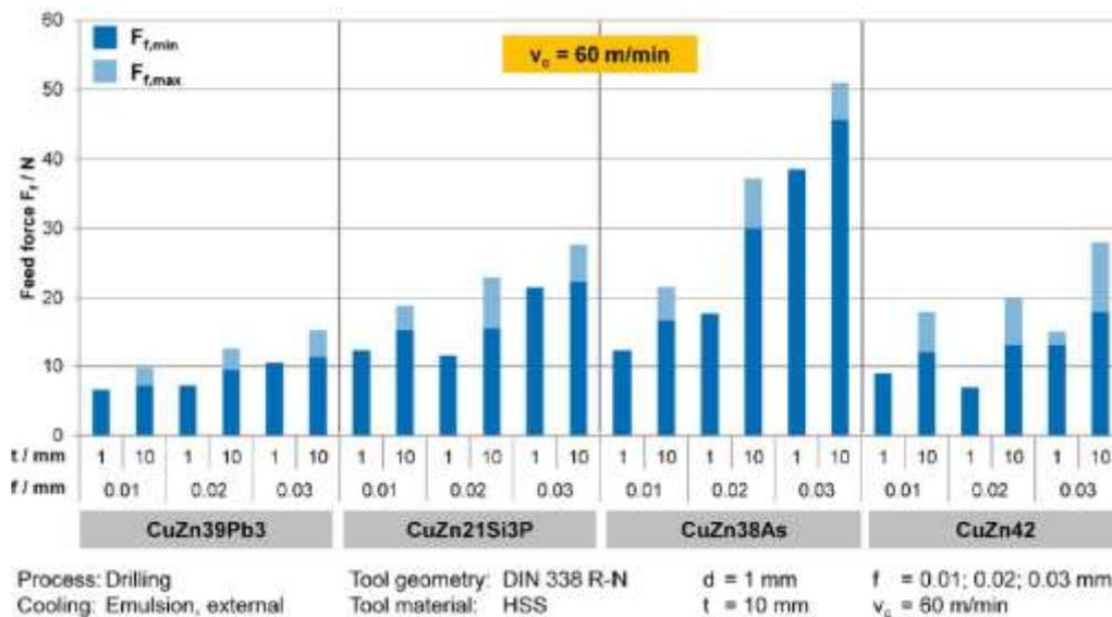
Fig. 14 Comparison of feed force at a cutting speed of V<sub>c</sub> 60 m/min
