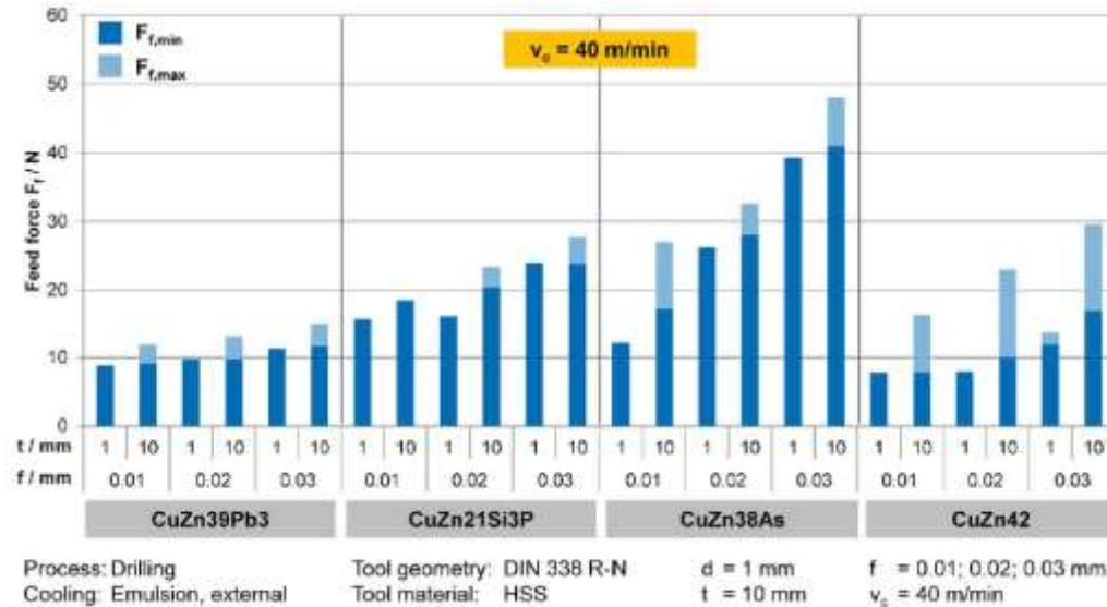
Fig. 13: Comparison of feed force at cutting speed of 40 m/min
