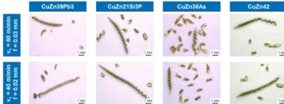
Fig. 10: Examples of long chips observed
