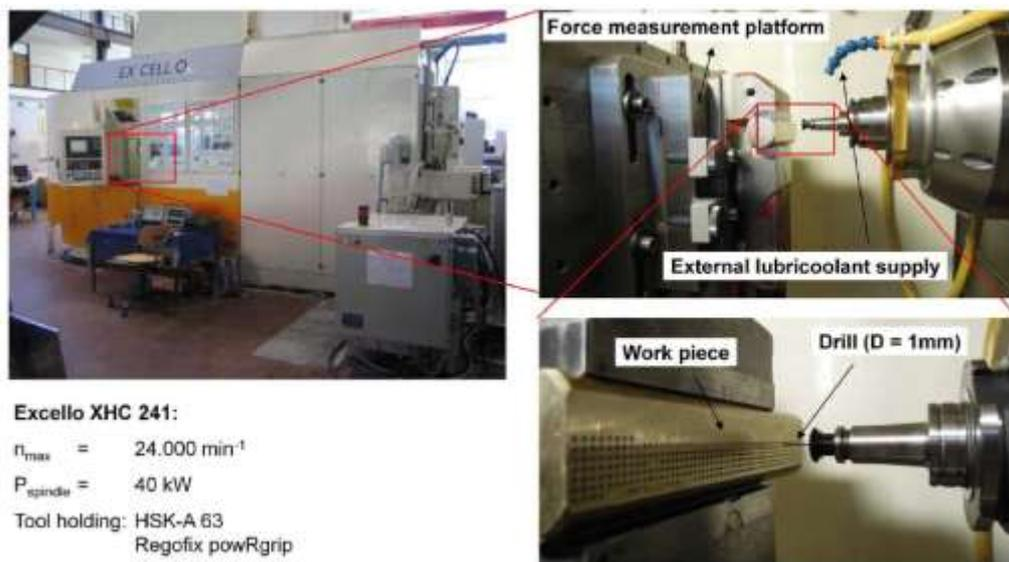
Figure 1: Experiment setup on Excello type XHC 241
