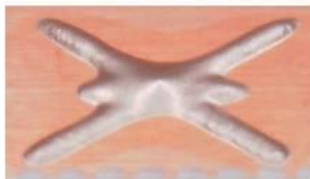
Dispense pattern with solvent bleed on the leadframe surface
