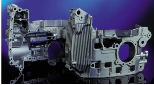
Picture 5: Aluminium pressure die casting Aluminium crankcase Material: AlSi9Cu3(Fe) (Source BMW)
