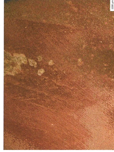
CW 713R – sample after the corrosion test – pitting and slight general corrosion
