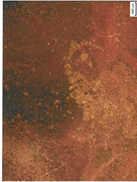
CW 713R – sample after the corrosion test – pitting and slight general corrosion
