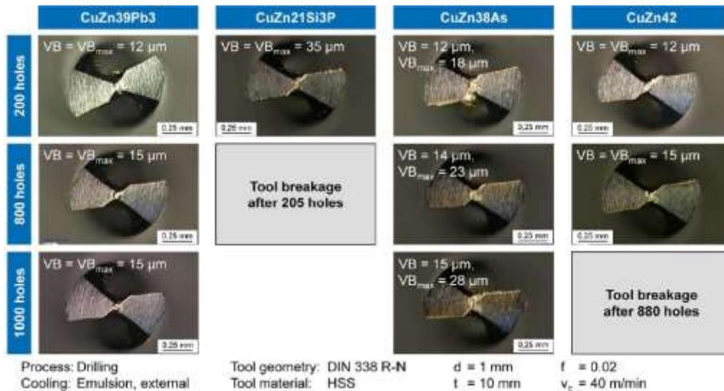
Fig. 17: Comparison of tool wear
