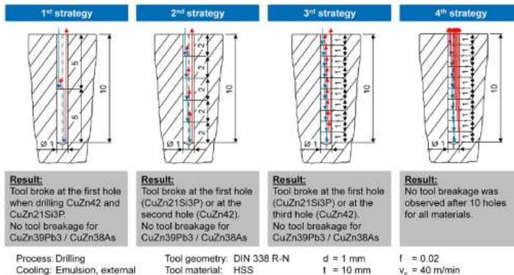
Figure 4: Investigation on the optimal drilling strategy
