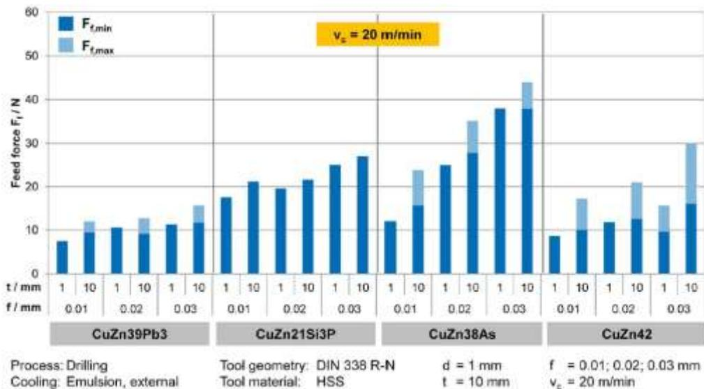
Fig. 12: Comparison of feed force at a cutting speed  $V_c$  of 20 m/min
