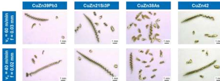
Fig. 10: Examples of long chips observed
