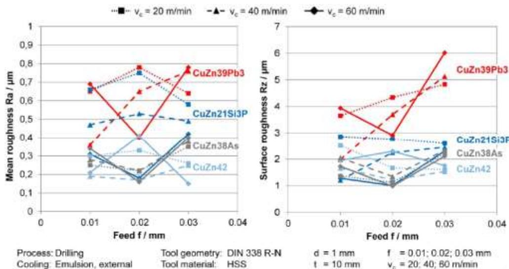
Fig. 15: Comparison of surface roughness
