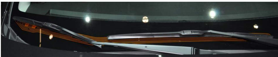
Figure 2: Windscreen wiper heating
