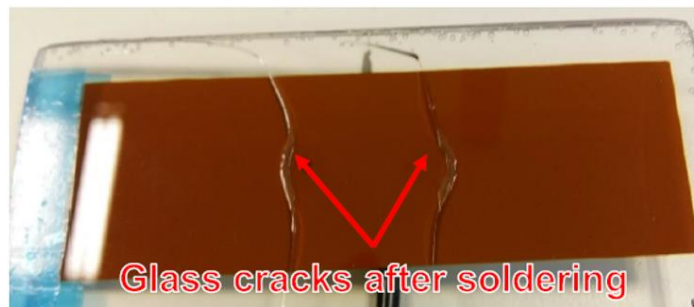
Figure 4: laboratory glass samples with soldered contact on surface
