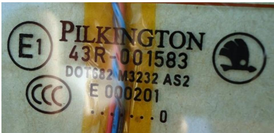
Figure 7: Skoda Octavia wagon - Backlite details
