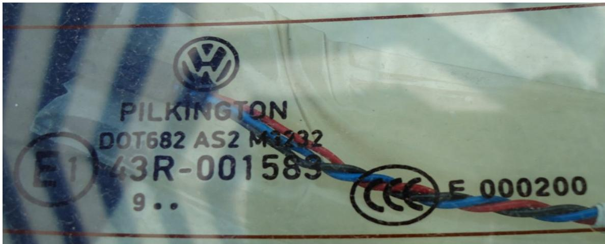
Figure 4: VW Eos Convertible - Backlite details
