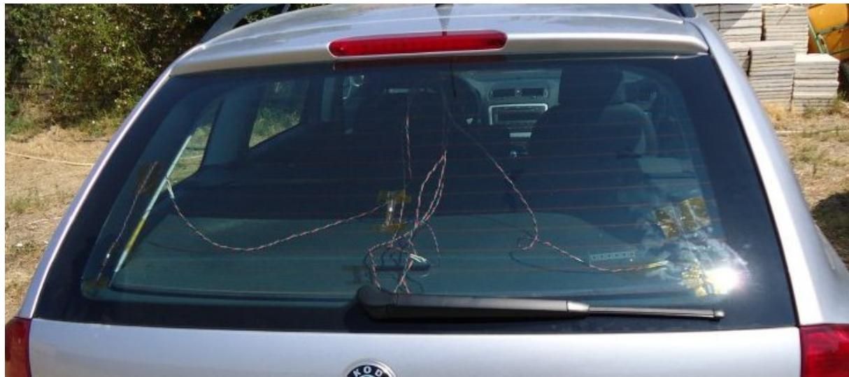
Figure 8: Skoda Octavia wagon - Sensor positioning
