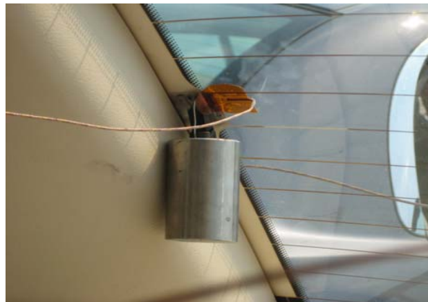
Ford backlite with thermocouple and .5kg weight
