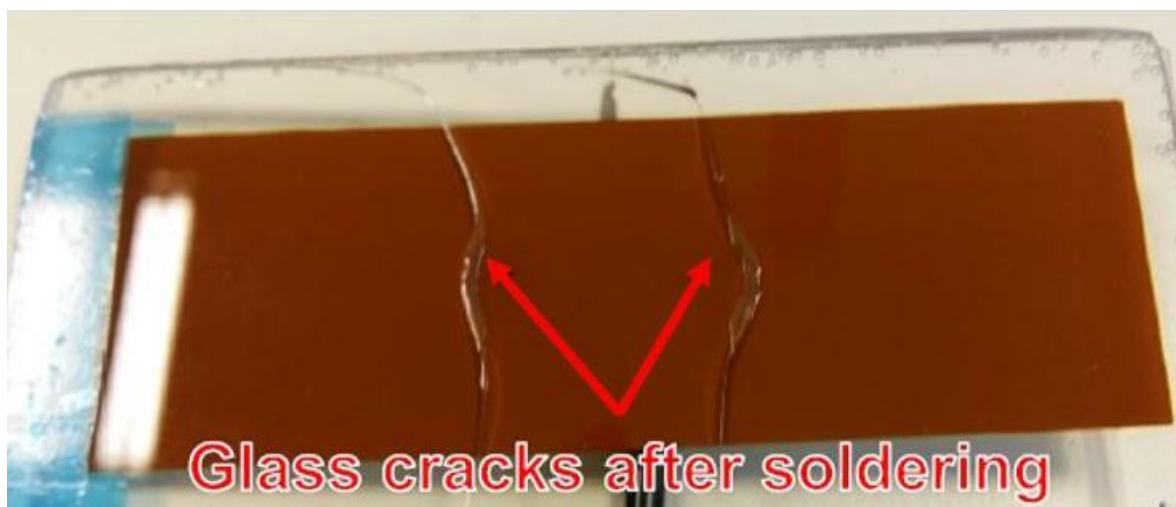
Figure 8-3: Cracked laboratory glass samples with soldered contact on surface 4
