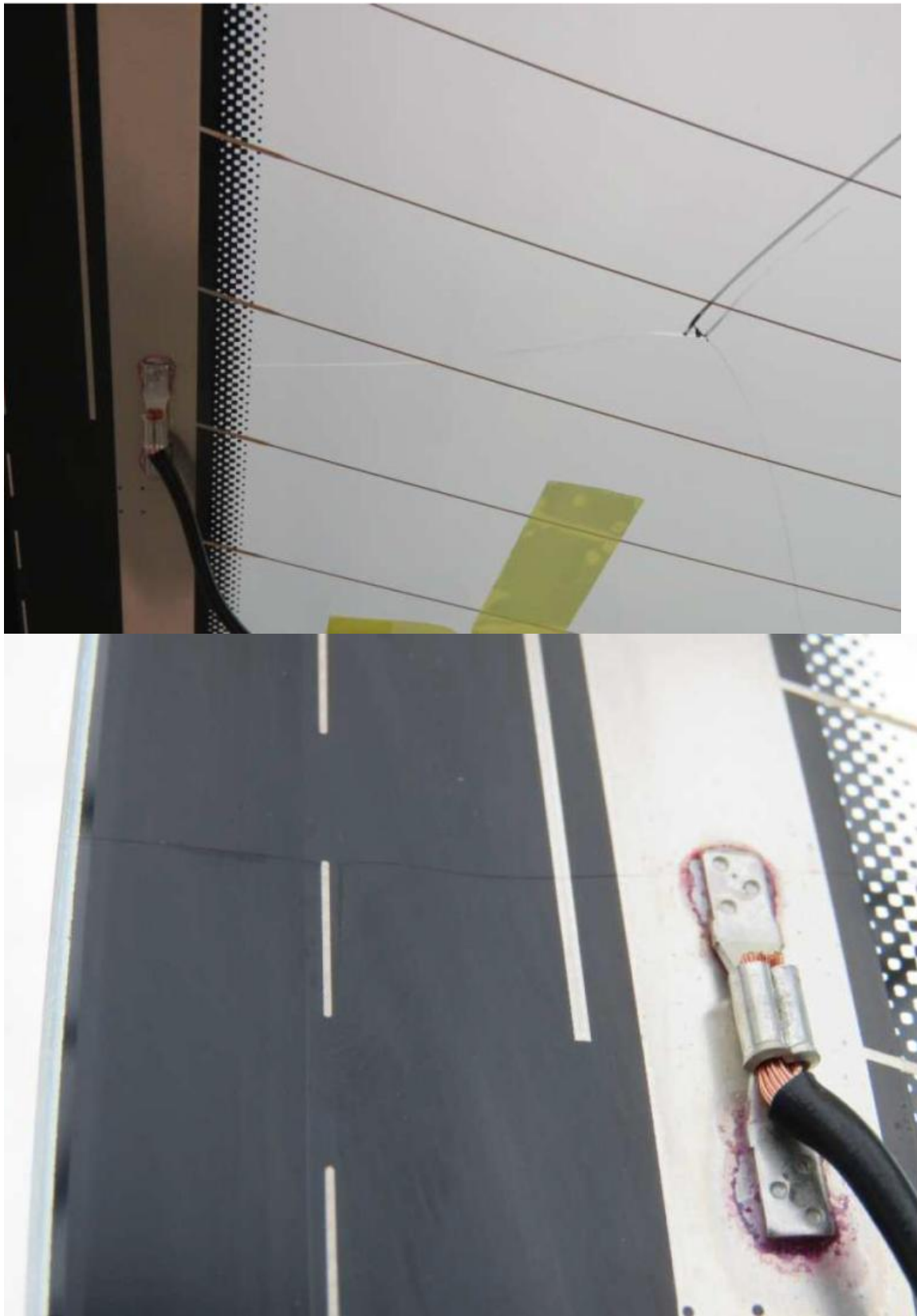
Figure 8-6: Lead-free soldered laminated backlights with glass breakages starting at the soldered bus bars
